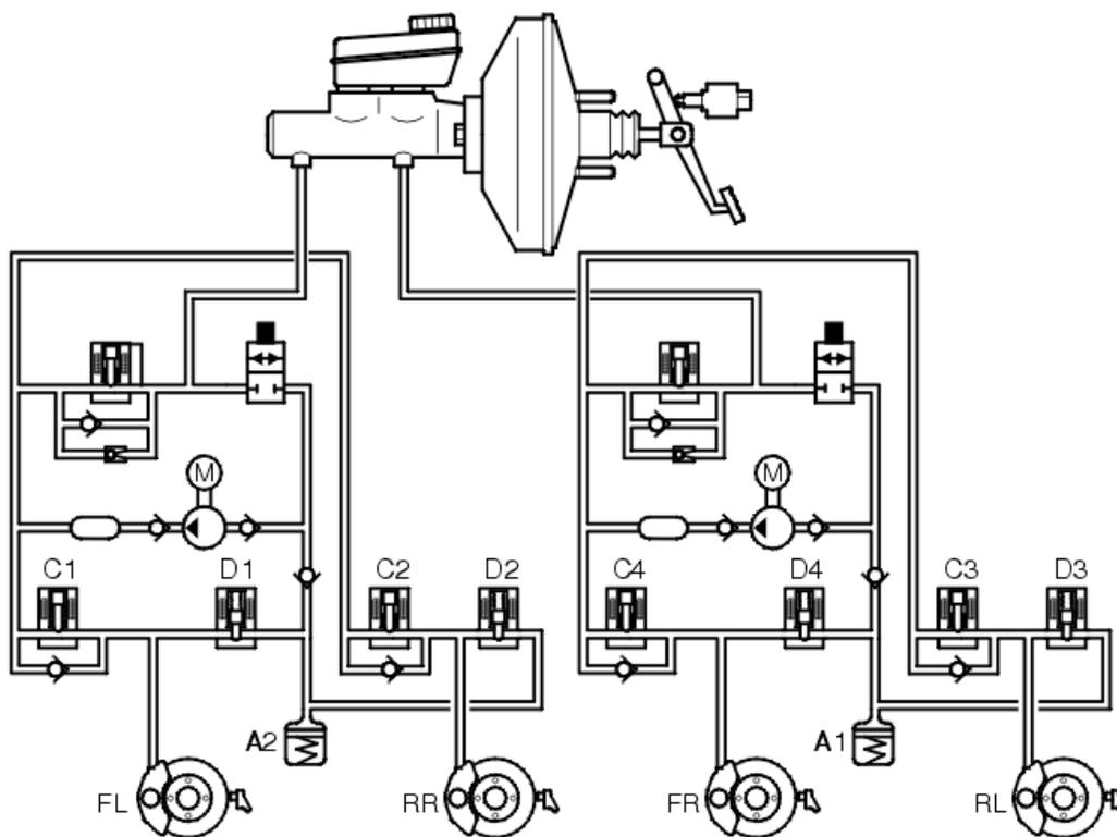
When the driven wheels are not spinning the brake system is unaffected (i.e. the master cylinder is in the rest position and the connections between the brake fluid reservoir and the rest of the hydraulic system are open). There is no pressure in the system. In the ABS hydraulic modulator valve block, the hydraulic valves are in their rest position. In other words, the inlet valves and the separation valves are open and the outlet valves closed.
