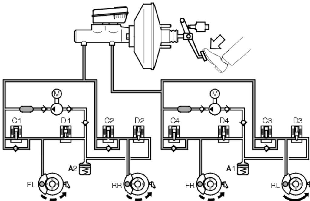
When a wheel locks-up under braking, the brake control module (BCM) begins to close the inlet valve for the relevant brake circuit so that the supply of brake fluid from the master cylinder is interrupted. This means that the hydraulic pressure cannot increase irrespective of the pressure in the master cylinder (constant pressure, see the right-hand front wheel - FR). The hydraulic pump starts at the same time.
