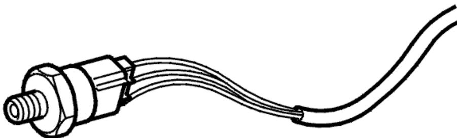
Two brake pressure sensors are positioned on the master cylinder. One sensor is located on the primary circuit and one on the secondary circuit. The information is transmitted via two analogue signals (measurement range 0-5 V) and is used by the brake control module (BCM) to calculate the brake pressure during active yaw control, and when the driver applies the brakes.
