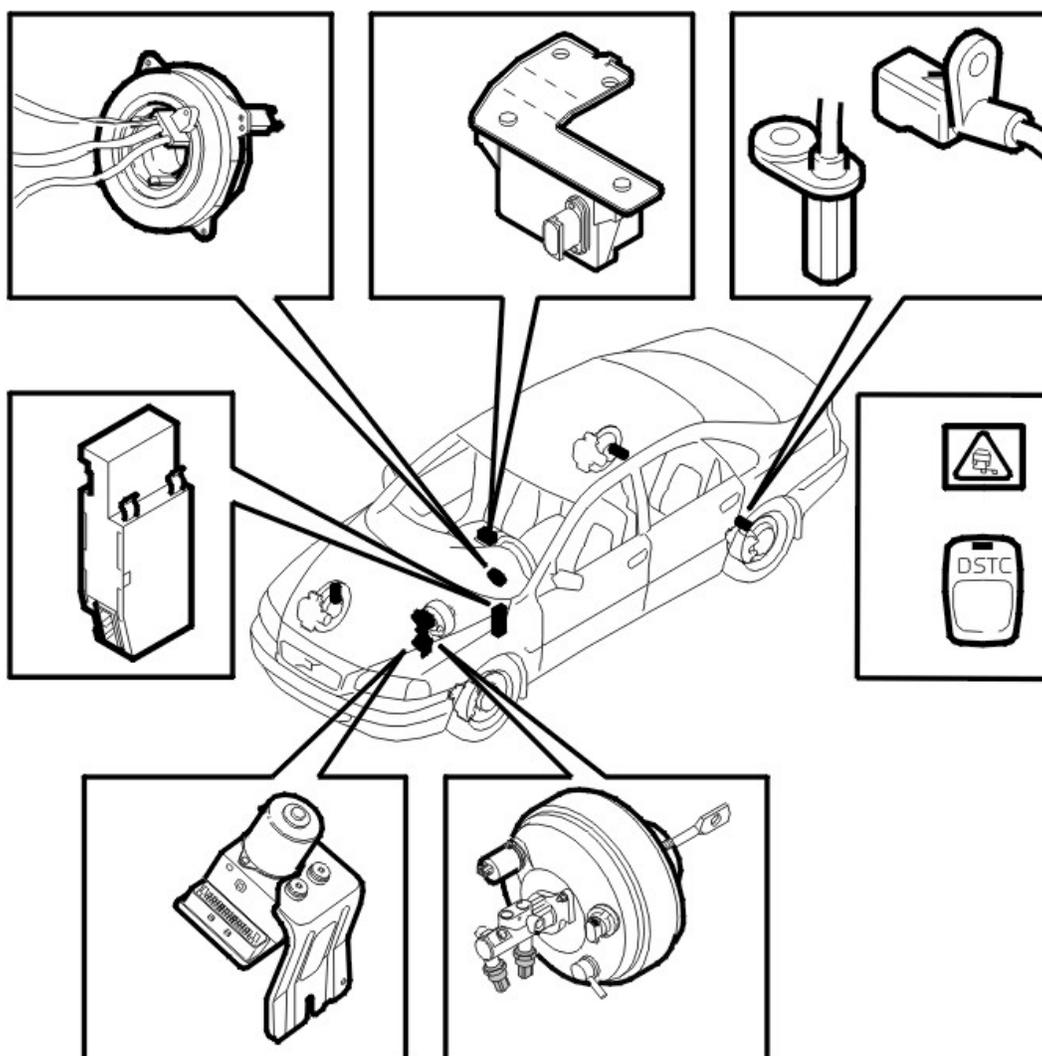
The brake control module (BCM) with DSTC (dynamic stability and traction control) uses continuous information from the different
