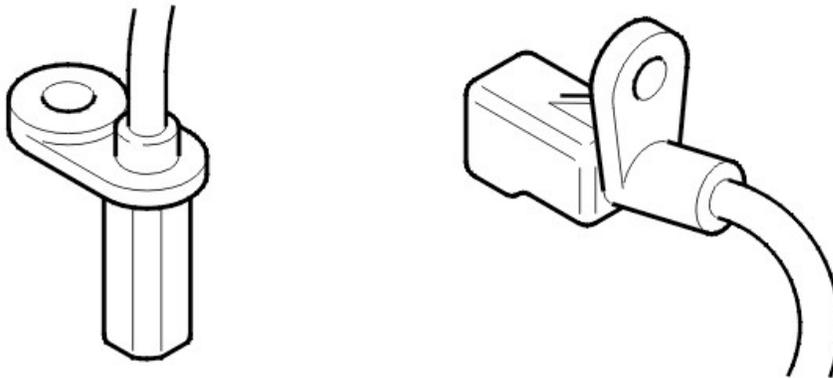
There are four wheel sensors, one at each wheel. The wheel sensors supply the control module with information about the rotation speed, acceleration and retardation of each wheel. By recording the pulses, the control module can calculate the wheel speed.
