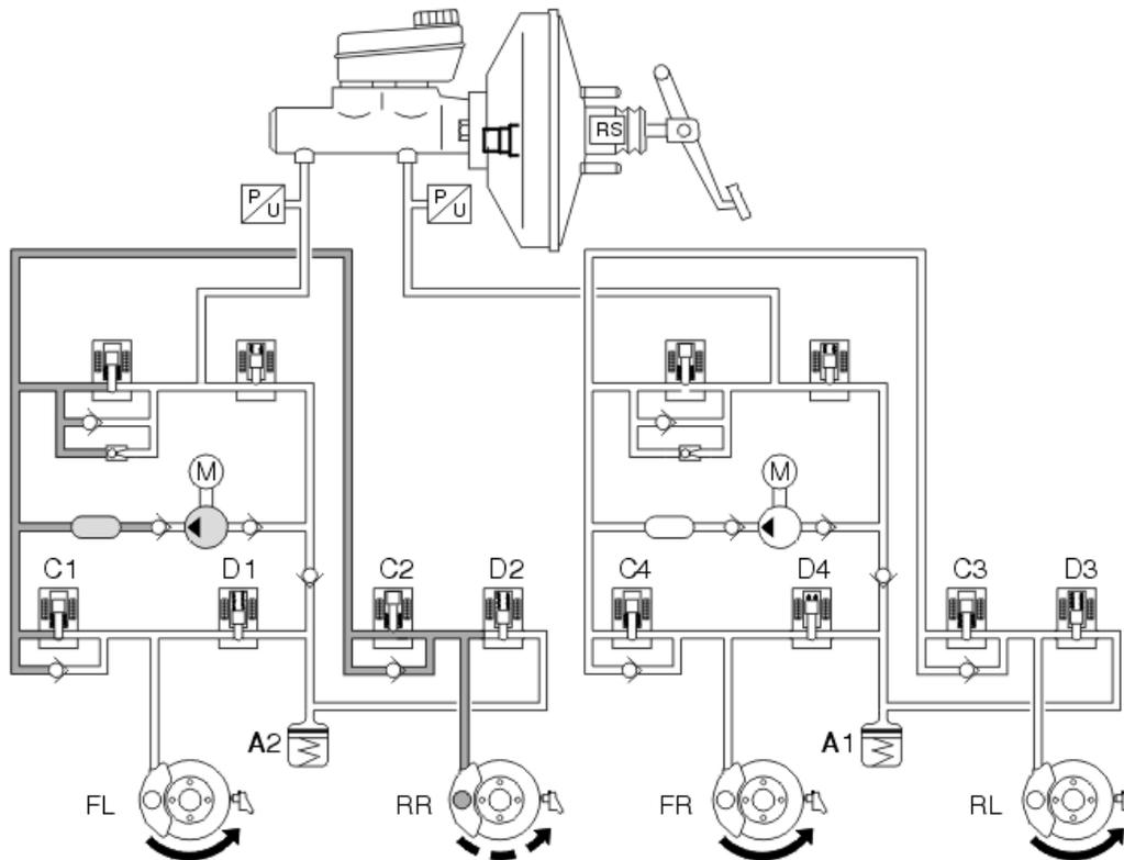
Understeer is when the car continues straight forward even though the steering wheel has been turned. Understeer is caused by too much acceleration. When the car understeers the brake control module (BCM) transmits a request for torque reduction to the engine control module (ECM) via the Controller area network (CAN).
