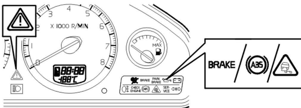
The brake system uses four warning lamps positioned in the combined instrument panel.
